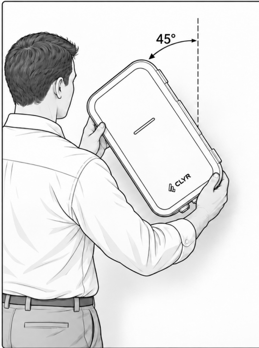
3 Tilt 45° counterclockwise and engage
