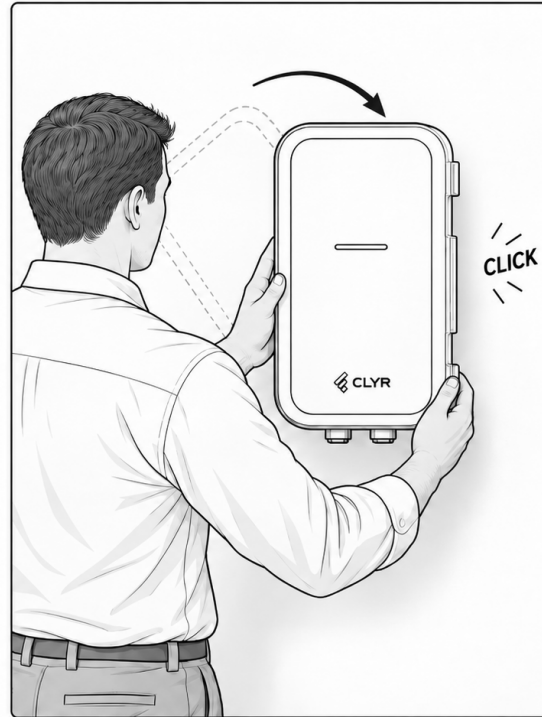
4 Turn clockwise until upright and locked
